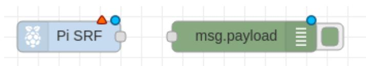
Double click the “rpi srf” node to open its configuration settings. Set **Pins** to “16,18” (which correspond to GPIO 23,24). The programmer of this node decided that it was better to use the Raspberry Pi’s board pinout rather than the BCM standard, [this](#) web page shows both.
